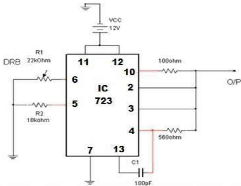
**FIG: LOW DROP OUT (LDO) REGULATOR USING 723 IC**
