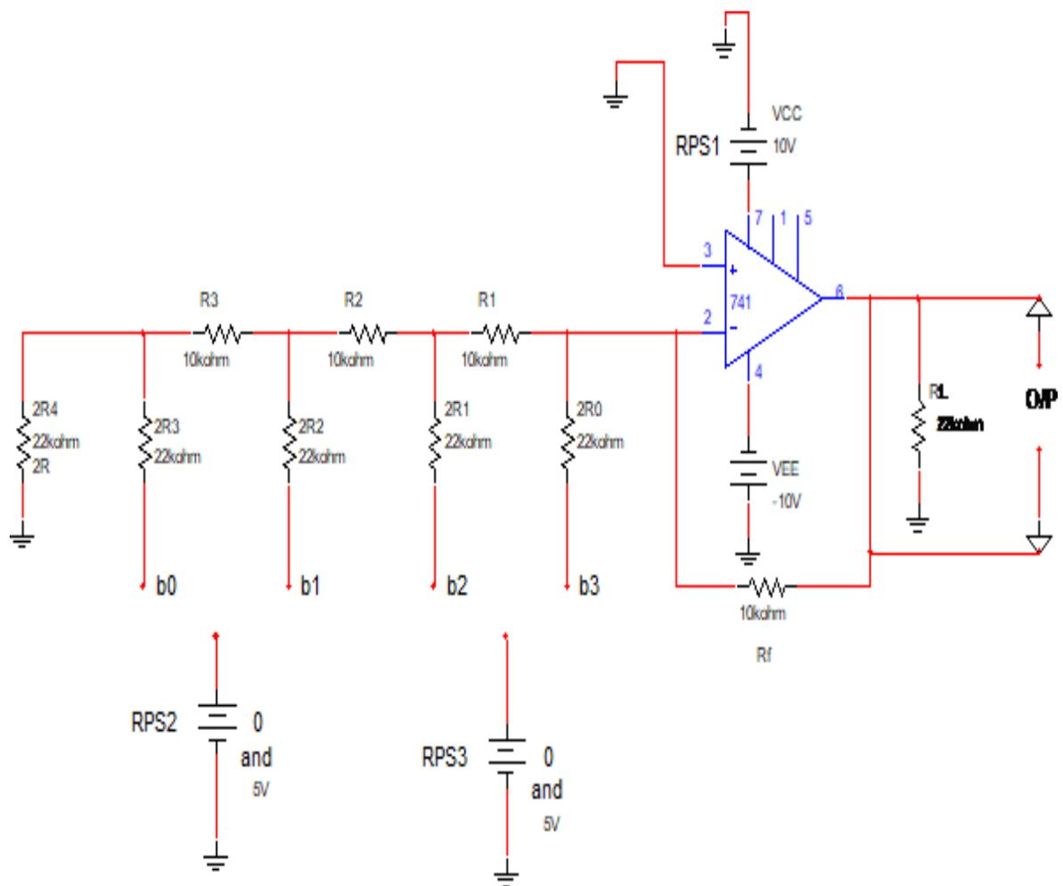
**FIG: 4-BIT D TO A CONVERTER**
