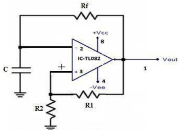
**FIG: ASTABLE MULTIVIBRATOR****PROCEDURE:**
