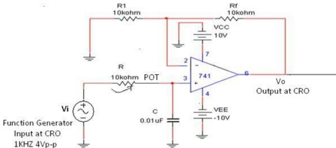
FIG: LOW PASS FILTER USING 741 I.C.
