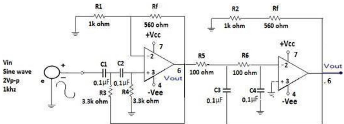
FIG: ANALOG FILTER-I
