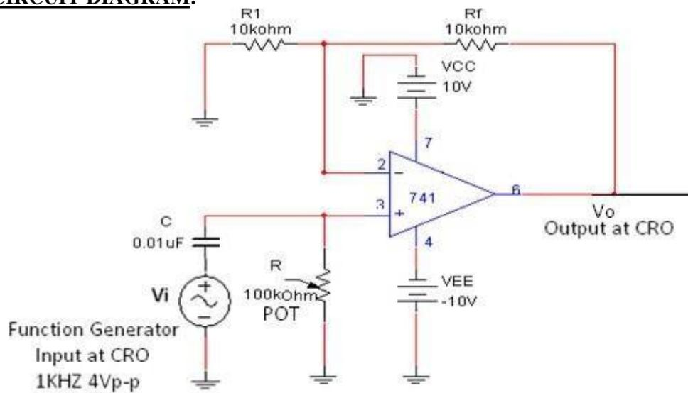
FIG: HIGH PASS FILTER USING 741 I.C.
