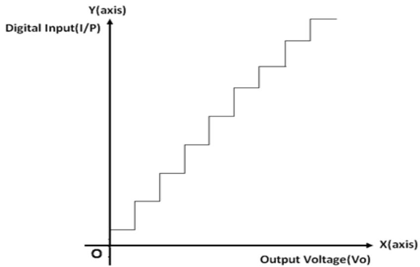
**FIG: 4-BIT D/A CONVERTER****RESULT:**
