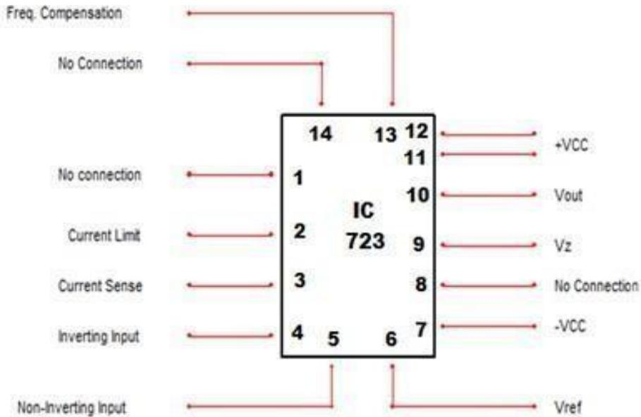
**FIG: PIN DIAGRAM OF LOW DROP OUT(LDO) REGULATOR USING 723 IC****CIRCUIT DIAGRAM:**
