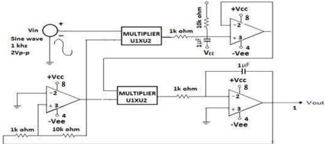
FIG: DESIGN OF A PHASE LOCKED LOOP
