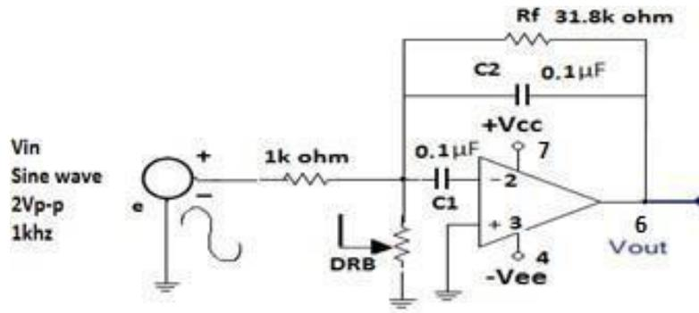
FIG: NARROW BANDPASS FILTER
